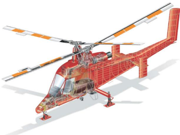
The K-MAX helicopter is about to enter a new realm of safety and performance as an optionally piloted UAS that can be configured to conduct a multi tasks with its outstanding and useful payload of 6,000 pounds.
