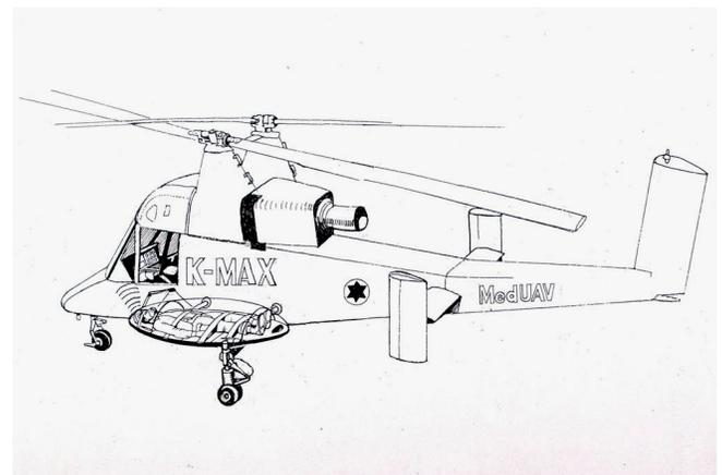
Fisher external MLSTAT payload MedEvac configuration, may enhance the potential for appropriate first responder care and evacuation, performed by combat medics, during the so called "Golden Hour" of combat casualty care, utilizing the benefits and new abilities of the MLSTAT solution designed currently by MedUAV partners.
